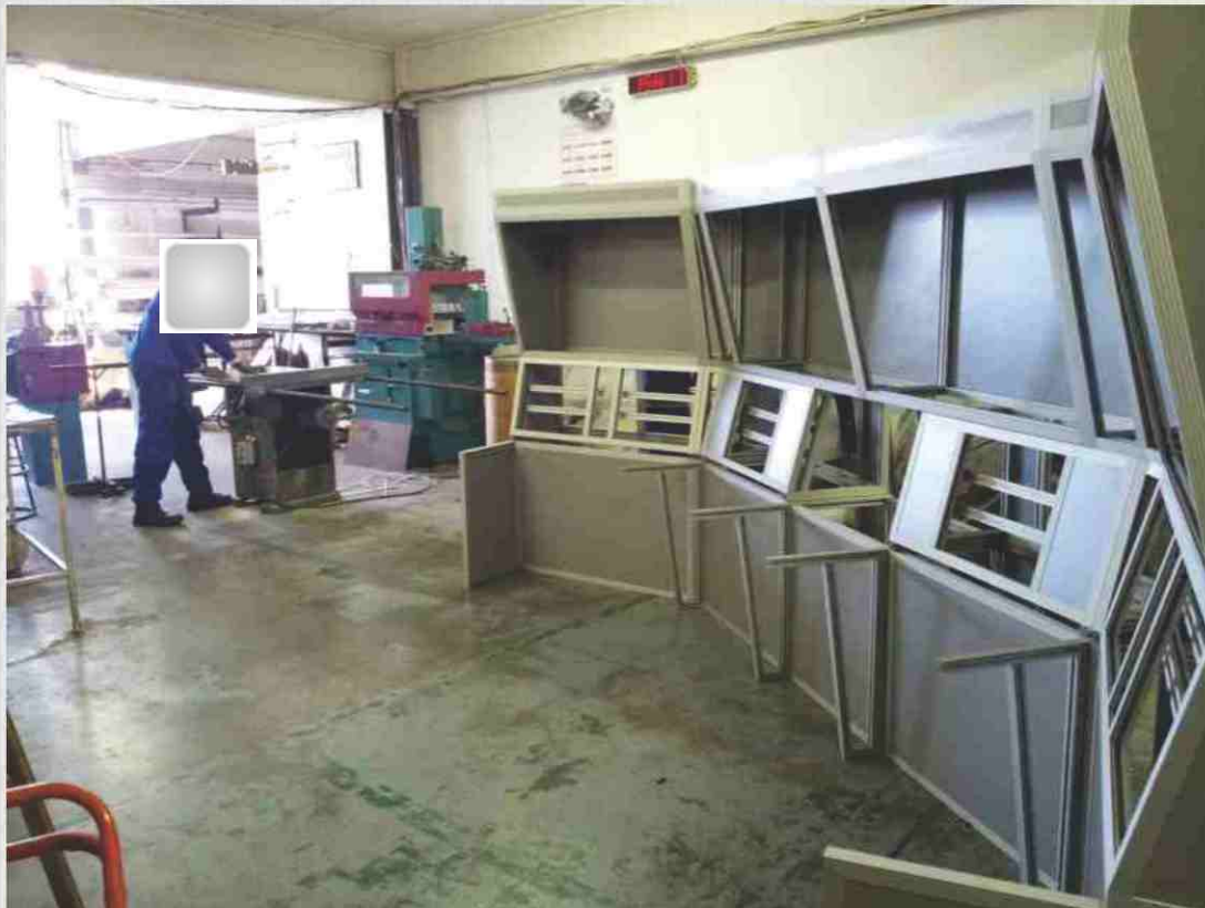
Above shows part of factory showing ALUTECH control desk under construction with one of our Control Room Clocks on the wall behind.
