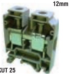
KUT 25 1000V/101A/25sq mm/2.3Nm
