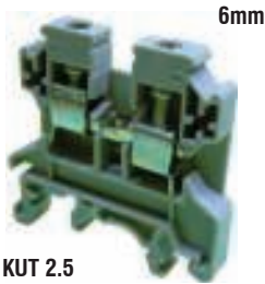
KUT 2.5 800V/24A/2.5sq mm/0.5Nm
