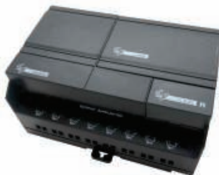
SR-22MRAC (22 I/O PLC UNIT) 14 Point AC or DC digital Inputs 8 point relay outputs 8 point transistor outputs (NPN / PNP)
