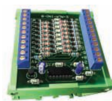
SASB....SIMPLE ALARM CARD 8 WAY
