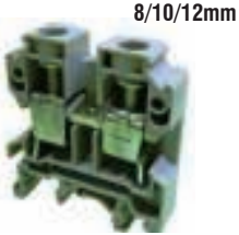
KUT6/10/16 800V/41A/6sq mm/0.8Nm 800V/57A/10sq mm/1.2Nm 800V/76A/16sq mm/1.2Nm
